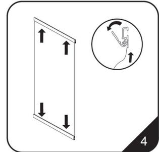
4. Swing open the beam's locking lip in order to attach the top & bottom edge of the banner. (Make sure the front of the banner is on the same side as the lip).
