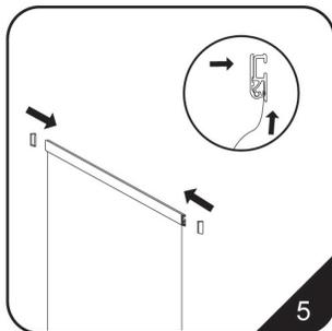
5. Slide the top banner edge under the lip. (if should go in about 3/8" or 1 cm) and close the lip to secure the banner. (same process for the bottom beam)
