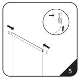
5. Slide the top banner edge under the lip.(if should go in about 3/89 or 1 cm) and close the lip to secure the banner.(same process for the bottom beam)
