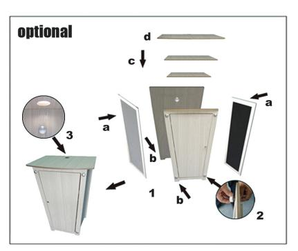
Install the roof printing and supporting profile.
