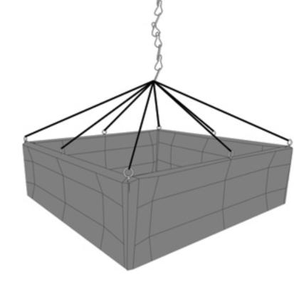
7. PLACE THE FABRIC ON EACH CORNER. REMOVE THE SCREW AND REPLACE WITH EYE HOOK. THEN PROCEED WITH THE REST OF THE BANNER. THEN ZIP UP INNER FABRIC. 8. USE CABLE THROUGH EYE HOOKS. TIGHTEN WITH HOOK LOOP LOCK. USE CABLE TO HOOK THROUGH CHAINS ON SUPPORTING STRUCTURES. ALSO EXTRA PARTS MAY BE NEEDED FOR CUSTOM HANGING.
