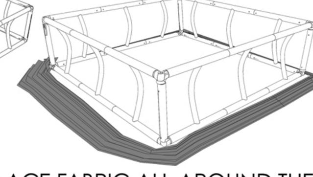
5. START TO CONNECT THE CURVED STABILIZER WITH LARGE SCREWS. ONE ON THE BOTTOM
